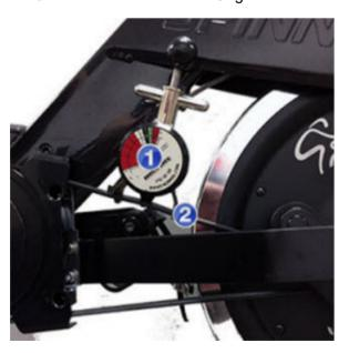
4. Adjust the belt tension between 140 - 150 lbs tension using the 13 mm belt tensioner adjustment nut
